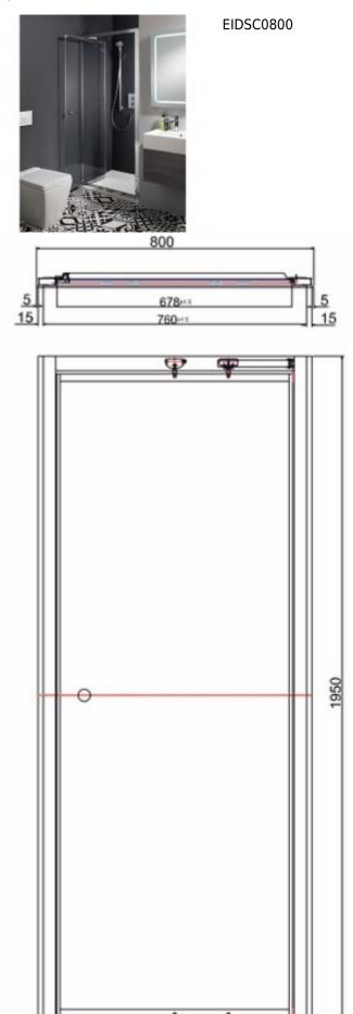
Note: Whole dimension tolerance is ±5. Glass dimension tolerance is ±2.
