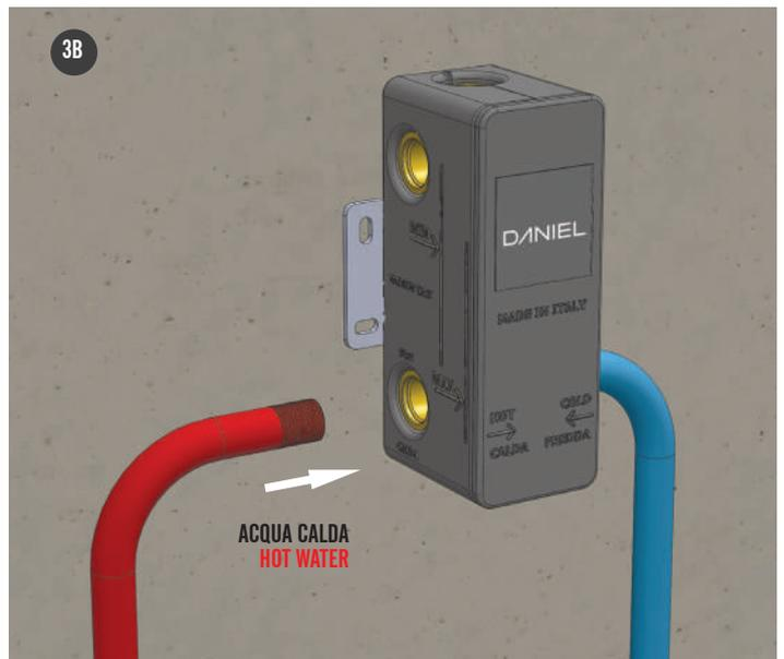
*Connect the cold (3A) and hot (3B) water pipes following the instructions printed on the built-in box.*
