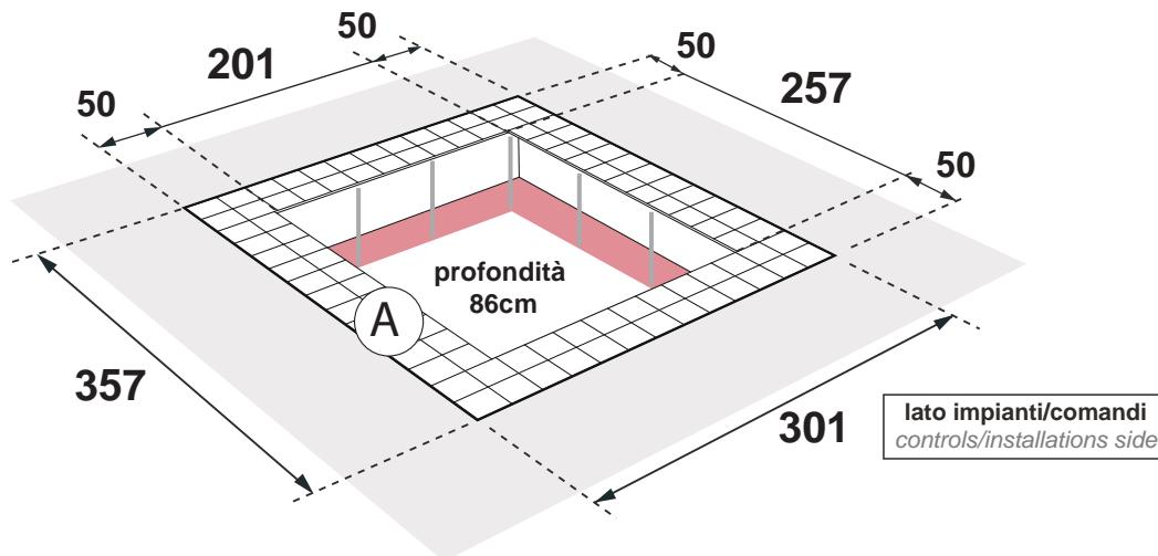
**A) DETTAGLI VANO INCASSO / INSPECTION COMPARTMENT DETAILS**
